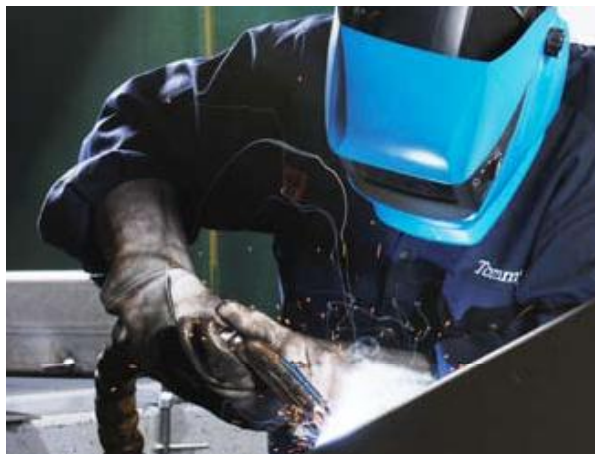
Welding torch with integrated fume extraction
